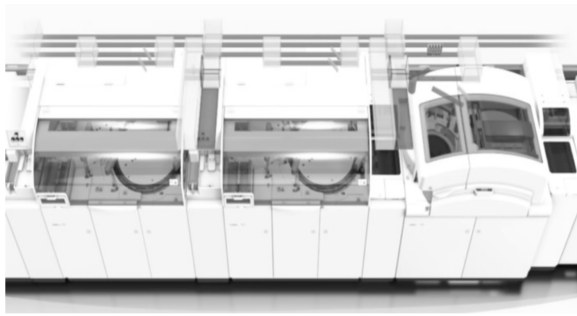
Fig. 2. Automated laboratory [52] with internal transportation system based on conveyor belts
